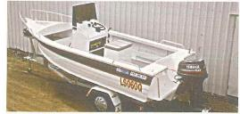
MATERIAL: Bottom 3mm & Sides 2mm BEAM: 2.1m DEPTH: 1.1m NUMBER OF FLOOR RIBS: 14 WEIGHT APPROX.: 380kg MAX Hp: 90
