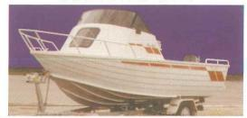
MATERIAL: Bottom 3mm & Sides 2mm BEAM: 2.2m DEPTH: 1.1m NUMBER OF FLOOR RIBS: 14 WEIGHT APPROX.: 485kg MAX Hp: 115
