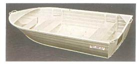
MATERIAL: Bottom & Sides 1.6m BEAM: 1.55m DEPTH: .64m NUMBER OF FLOOR RIBS: 7 WEIGHT APPROX.: 80kg MAX Hp: 20
